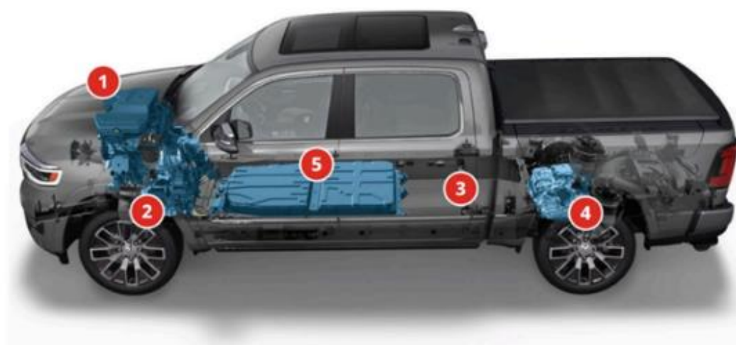
FIGURE 41: THE ANATOMY OF A RANGE-EXTENDED ELECTRIC VEHICLE
